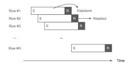
Figure 1: CMOS image sensor operation with rolling shutter.
